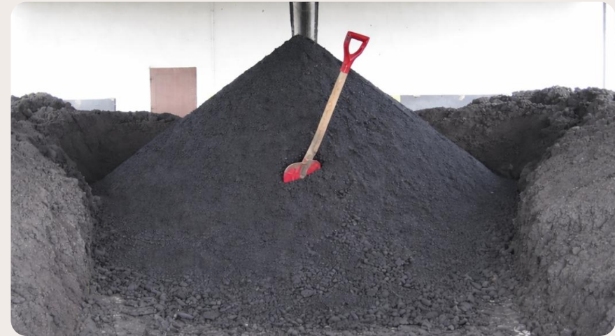
Biosolids with thermal hydrolysis treatment
